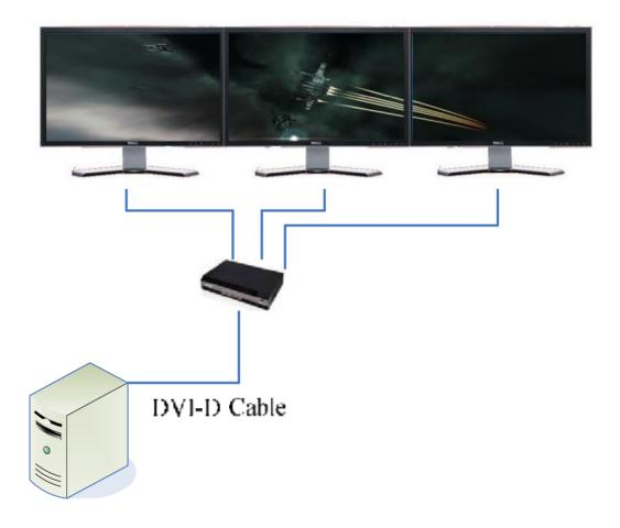
Figure 3 Typical application of Triple-monitors wide screen
